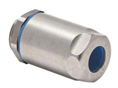
Bimed hygienic EMC cable gland, M16 x 1.5mm thread type, stainless steel, accepts 5 to 10mm diameter cable, IP66, IP68 and IP69. Mounting hardware included. Allen wrench size 10mm, use adapter BMFGT-02 to reduce Allen wrench size to 6mm.
