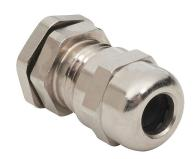
Bimed cable gland, M12  $\times$  1.5mm thread type, nickel-plated brass, accepts 3 to 6.5mm diameter cable, IP68. Package of 5. Mounting hardware included.
