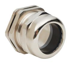
Bimed cable gland, M63 x 1.5mm thread type, nickel-plated brass, accepts 34 to 44mm diameter cable, IP68. Package of 2. Mounting hardware included.
