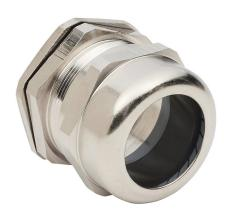
Bimed cable gland, M50  $\times$  1.5mm thread type, nickel-plated brass, accepts 27 to 38mm diameter cable, IP68. Package of 2. Mounting hardware included.
