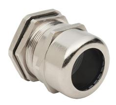
Bimed cable gland, M40 x 1.5mm thread type, nickel-plated brass, accepts 19 to 28mm diameter cable, IP68. Package of 2. Mounting hardware included.
