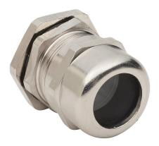
Bimed cable gland, M25 x 1.5mm thread type, nickel-plated brass, accepts 11 to 17mm diameter cable, IP68. Package of 5. Mounting hardware included.
