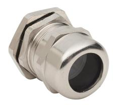
Bimed cable gland, M25  $\times$  1.5mm thread type, nickel-plated brass, accepts 11 to 17mm diameter cable, IP68. Package of 5. Mounting hardware included.
