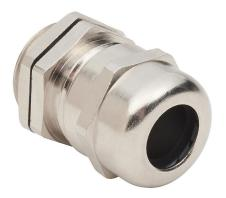
Bimed cable gland, M20 x 1.5mm thread type, nickel-plated brass, accepts 6 to 12mm diameter cable, IP68. Package of 5. Mounting hardware included.
