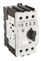
Fuji Electric BM3V series manual motor protector, rotary, 63A, thermal overload, 45.0-63.0A adjustable, 819A instantaneous trip rating, open, 55mm frame.
