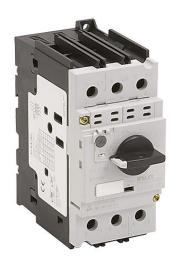
Fuji Electric BM3V series manual motor protector, rotary, 50A, thermal overload, 35.0-50.0A adjustable, 650A instantaneous trip rating, open, 55mm frame.
