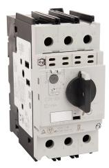
Fuji Electric BM3V series manual motor protector, rotary, 32A, thermal overload, 24.0-32.0A adjustable, 416A instantaneous trip rating, open, 55mm frame.
