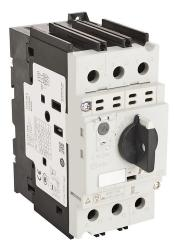
Fuji Electric BM3V series manual motor protector, rotary, 25A, thermal overload, 19.0-25.0A adjustable, 325A instantaneous trip rating, open, 55mm frame.
