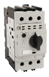
Fuji Electric BM3V series manual motor protector, rotary, 20A, thermal overload, 14.0-20.0A adjustable, 260A instantaneous trip rating, open, 55mm frame.
