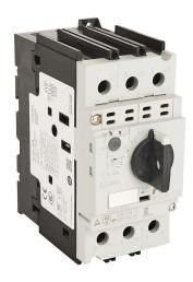
Fuji Electric BM3V series manual motor protector, rotary, 16A, thermal overload, 11.0-16.0A adjustable, 208A instantaneous trip rating, open, 55mm frame.
