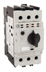
Fuji Electric BM3V series manual motor protector, rotary, 13A, thermal overload, 9.0-13.0A adjustable, 169A instantaneous trip rating, open, 55mm frame.
