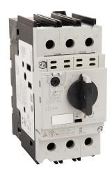
Fuji Electric BM3V series manual motor protector, rotary, 10A, thermal overload, 6.3-10.0A adjustable, 130A instantaneous trip rating, open, 55mm frame.
