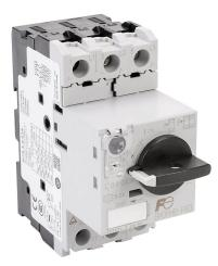
Fuji Electric BM3R series manual motor protector, rotary, 0.63A, thermal overload, 0.4-0.63A adjustable, 8.2A instantaneous trip rating, open, 45mm frame.
