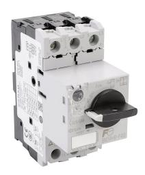
Fuji Electric BM3R series manual motor protector, rotary, 0.4A, thermal overload, 0.25-0.4A adjustable, 5.2A instantaneous trip rating, open, 45mm frame.
