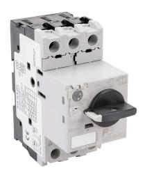
Fuji Electric BM3R series manual motor protector, rotary, 0.25A, thermal overload, 0.16-0.25A adjustable, 3.3A instantaneous trip rating, open, 45mm frame.
