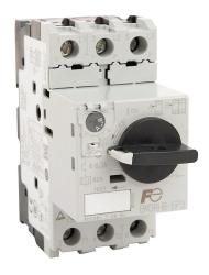
Fuji Electric BM3R series manual motor protector, rotary, 6.3A, thermal overload, 4.0-6.3A Adjustable, 81.9A instantaneous trip rating, open, 45mm frame.
