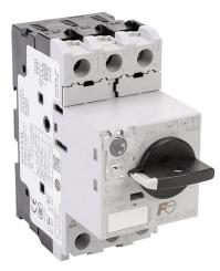
Fuji Electric BM3R series manual motor protector, rotary, 2.5A, thermal overload, 1.6-2.5A adjustable, 32.5A instantaneous trip rating, open, 45mm frame.
