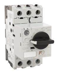
Fuji Electric BM3R series manual motor protector, rotary, 1.6A, thermal overload, 1.0-1.6A adjustable, 20.8A instantaneous trip rating, open, 45mm frame.
