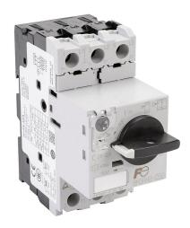
Fuji Electric BM3R series manual motor protector, rotary, 32A, thermal overload, 24.0-32.0A adjustable, 416A instantaneous trip rating, open, 45mm frame.
