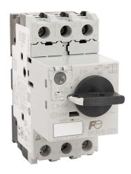
Fuji Electric BM3R series manual motor protector, rotary, 25A, thermal overload, 19.0-25.0A adjustable, 325A instantaneous trip rating, open, 45mm frame.
