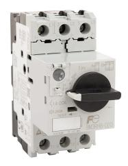
Fuji Electric BM3R series manual motor protector, rotary, 20A, thermal overload, 14.0-20.0A adjustable, 260A instantaneous trip rating, open, 45mm frame.
