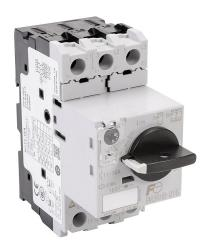
Fuji Electric BM3R series manual motor protector, rotary, 16A, thermal overload, 11.0-16.0A adjustable, 208A instantaneous trip rating, open, 45mm frame.
