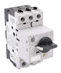
Fuji Electric BM3R series manual motor protector, rotary, 13A, thermal overload, 9.0-13.0A adjustable, 169A instantaneous trip rating, open, 45mm frame.
