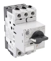
Fuji Electric BM3R series manual motor protector, rotary, 10A, thermal overload, 6.3-10.0A adjustable, 130A instantaneous trip rating, open, 45mm frame.
