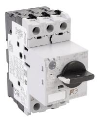
Fuji Electric BM3R series manual motor protector, rotary, 4A, thermal overload, 2.5-4.0A adjustable, 52A instantaneous trip rating, open, 45mm frame.
