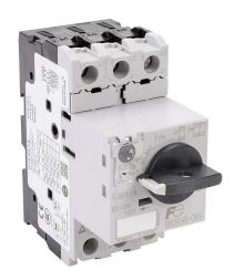
Fuji Electric BM3R series manual motor protector, rotary, 1A, thermal overload, 0.63-1.0A adjustable, 13A instantaneous trip rating, open, 45mm frame.
