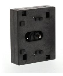
AutomationDirect mechanical interlock, for use with GH15BN, GH15CN, GH15DN, GH15ET, GH15FT GH15GT, GH15HT, GH15JT, GH15KT, GH15LT or GH15MT series contactors, mechanically connects contactors to prevents both from being pulled in at the same time.
