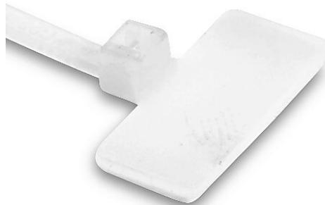
Identification nylon 6.6 cable tie, 4in length, 0.09in width, 18 lb tensile strength, 0.7in maximum bundle diameter, natural, (1) 0.8 x 0.35in top mounted transversal ID tag. Package of 100.
