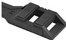
UV resistant nylon 12 cable tie, 14in length, 0.35in width, 112 lb tensile strength, 3.66in maximum bundle diameter, black. Package of 100.
