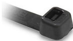
Nylon 6.6 cable tie, 11in length, 0.18in width, 50 lb tensile strength, 2.99in maximum bundle diameter, black. Package of 1000.
