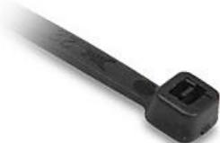
Nylon 6.6 cable tie, 11in length, 0.14in width, 40 lb tensile strength, 2.99in maximum bundle diameter, black. Package of 100.
