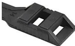
UV resistant nylon 12 cable tie, 10in length, 0.35in width, 112 lb tensile strength, 2.55in maximum bundle diameter, black. Package of 100.
