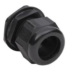
Bimed cable gland, M40 x 1.5mm thread type, polyamide, black, accepts 19 to 28mm diameter cable, IP68. Package of 2. Mounting hardware included.
