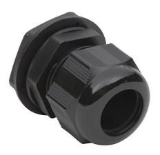
Bimed cable gland, M32 x 1.5mm thread type, polyamide, black, accepts 15 to 21mm diameter cable, IP68. Package of 5. Mounting hardware included.
