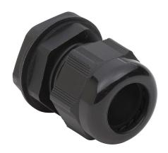
Bimed cable gland, M25 x 1.5mm thread type, polyamide, black, accepts 11 to 17mm diameter cable, IP68. Package of 5. Mounting hardware included.
