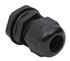
Bimed cable gland, M20 x 1.5mm thread type, polyamide, black, accepts 6 to 12mm diameter cable, IP68. Package of 5. Mounting hardware included.
