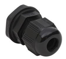
Bimed cable gland, M16 x 1.5mm thread type, polyamide, black, accepts 4 to 8mm diameter cable, IP68. Package of 5. Mounting hardware included.
