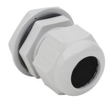
Bimed cable gland, M32 x 1.5mm thread type, polyamide, light gray, accepts 15 to 21mm diameter cable, IP68. Package of 5. Mounting hardware included.
