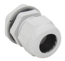
Bimed cable gland, M25 x 1.5mm thread type, polyamide, light gray, accepts 11 to 17mm diameter cable, IP68. Package of 5. Mounting hardware included.
