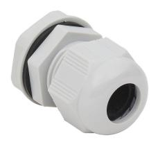
Bimed cable gland, M20 x 1.5mm thread type, polyamide, light gray, accepts 6 to 12mm diameter cable, IP68. Package of 5. Mounting hardware included.
