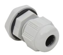
Bimed cable gland, M16 x 1.5mm thread type, polyamide, light gray, accepts 4 to 8mm diameter cable, IP68. Package of 5. Mounting hardware included.
