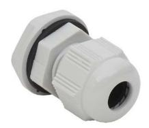
Bimed cable gland, M16 x 1.5mm thread type, polyamide, light gray, accepts 4 to 8mm diameter cable, IP68. Package of 5. Mounting hardware included.
