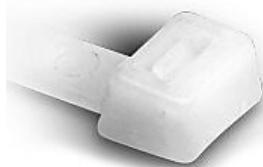
Nylon 6.6 cable tie, 14in length, 0.29in width, 120 lb tensile strength, 4.01in maximum bundle diameter, natural. Package of 100.
