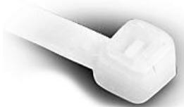
Nylon 6.6 cable tie, 11in length, 0.18in width, 50 lb tensile strength, 2.99in maximum bundle diameter, natural. Package of 100.
