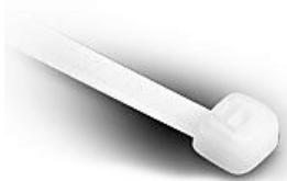
Nylon 6.6 cable tie, 8in length, 0.14in width, 40 lb tensile strength, 1.9in maximum bundle diameter, natural. Package of 1000.
