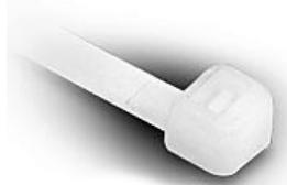
Nylon 6.6 cable tie, 7in length, 0.18in width, 50 lb tensile strength, 1.69in maximum bundle diameter, natural. Package of 1000.
