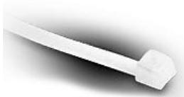
Nylon 6.6 cable tie, 6in length, 0.09in width, 18 lb tensile strength, 1.57in maximum bundle diameter, natural. Package of 1000.
