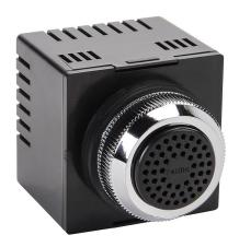
Patlite audible alarm buzzer, 90 dB at 1m, 3.9 kHz to 4.6 kHz tone frequency, (2) selectable tone(s), 120 VAC, 30mm, panel mount, ABS plastic housing, black, IP30.
